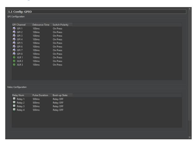
Use these configuration options to set the debounce times and polarity settings for the GPI inputs and pulse times for the GPO relays.
