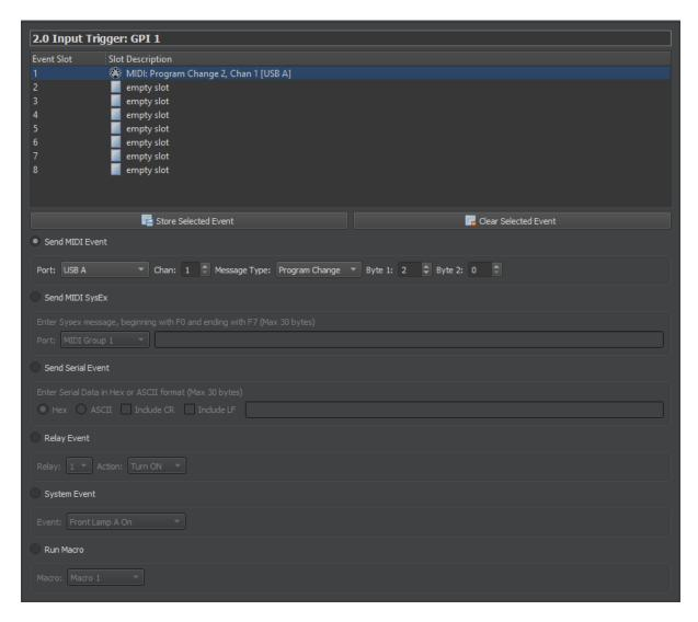
The CCS-2 has 11 configurable GPI input triggers, 8 are available on the 9-Pin D-Sub and a further 3 available as XLR connectors. These triggers are commonly used to perform cue operations such as Go, Stop, Previous, Next – sending MIDI data to playback software.
