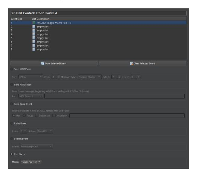
The 2 front panel switches and the 2 remote port switches can have up to 8 events or macros assigned to them, similar to the Input Triggers described above.
