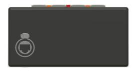
Power & Network – OSCA can be powered by POE IEEE 802.3 or 5v DC via the USB C port
