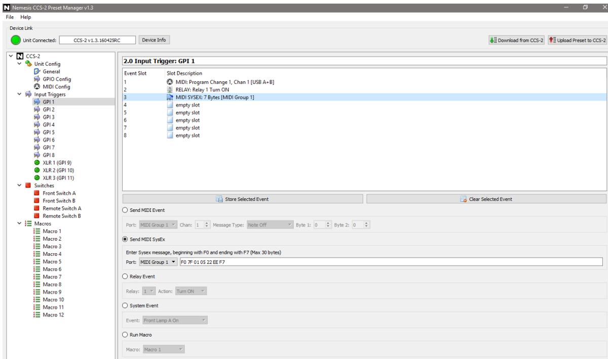
Available for Windows and MacOS, *Preset Manager* is the configuration utility for the CCS-2. The software allows most features of the CCS-2 to be user-configured, including the status of lamps, the effect of button pushes, MIDI routing strategies etc.
