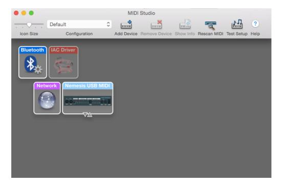
Once the device has been enumerated, OSX should install the device as a standard class compliant MIDI device. To check this has been successful, the device will be seen in the MIDI Studio (Window - > Show MIDI Window) part of Audio MIDI Setup found in Applications->Utilities.
