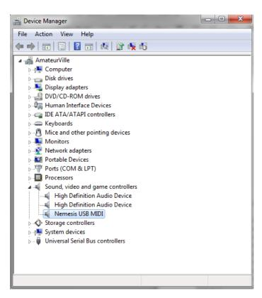
Windows 7/8/10 will detect the device and attempt to install it a standard USB MIDI device. It may connect to the internet to determine whether there is a driver to use other than the standard MIDI driver, but will be satisfied to use the standard class compliant driver.
