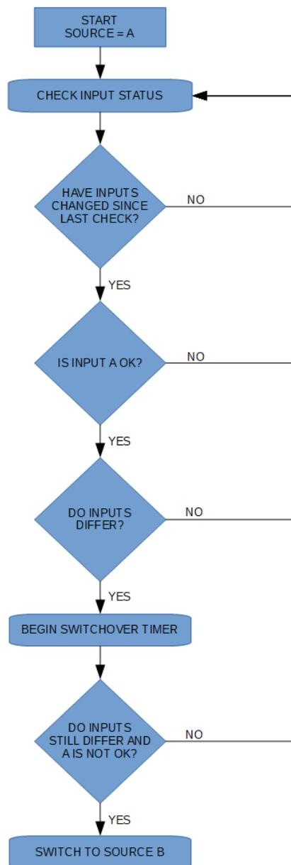
Once a fault has been detected and the ACS-PLUS has switched to the backup source, it will not automatically switch back to the primary source as this allows the user time to investigate the problem and be certain the source is reliable before/if running from this again. So in effect the above algorithm will sleep until it is manually switched back to A and the process begins over again. There are certain exceptions to this condition – see *Internal Options* for more information.
