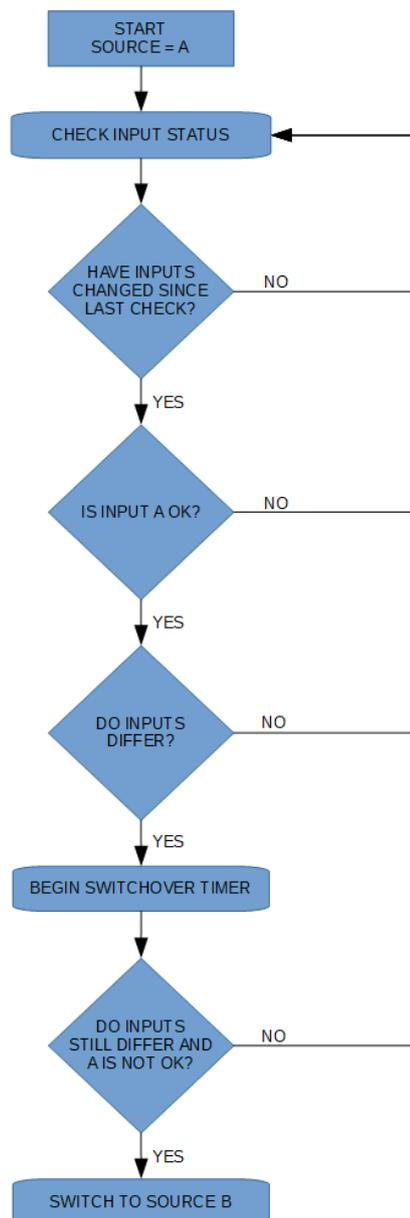
Once a fault has been detected and the ACS-1 has switched to the backup source, it will not automatically switch back to the primary source as this allows the user time to investigate the problem
