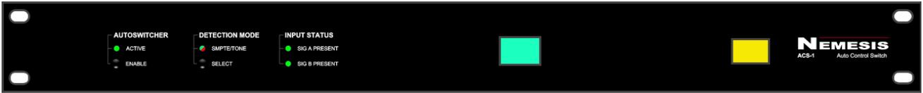
**The Nemesis ACS-1 Auto Switcher is a 1U rack mount unit that automatically controls any of the Nemesis range of switchover units by detecting the presence of playback signals using either a 1 kHz tone or SMPTE timecode.**
