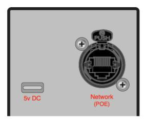
Power & Network – OSCA can be powered by POE or 5v DC via the USB C port
